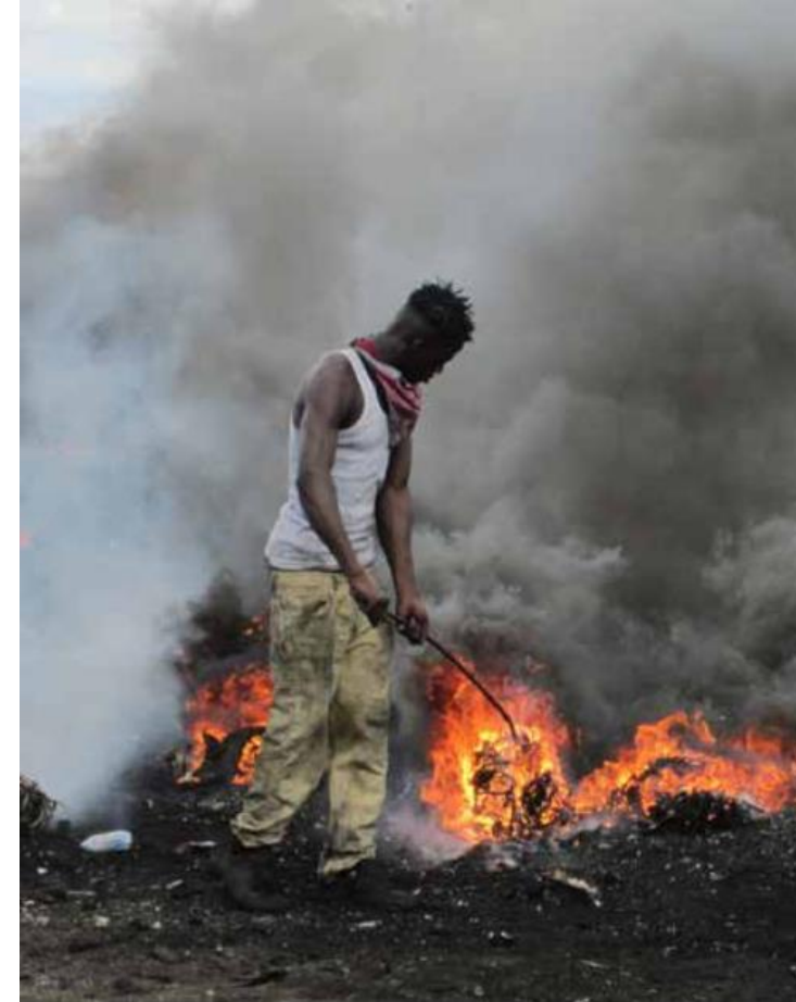
Recovery of copper from wires in open fire (Accra/Ghana; Source: Öko-Institut)
